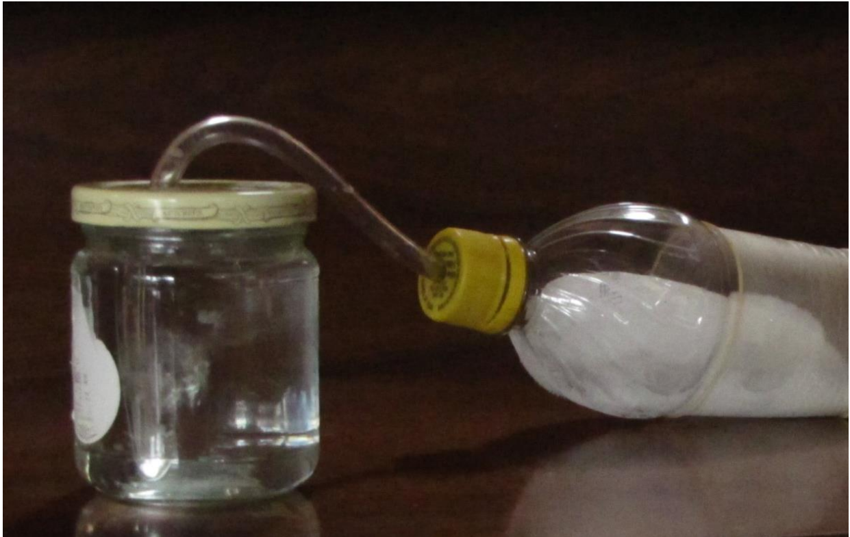
Fig. 1. The lab set-up mimicking how corals make calcium carbonate, using household equipment and readily obtainable materials. Dry ice in the plastic bottle supplies carbon dioxide through the straw into the glass jar of ocean water surrogate bought from a pet store. Clear sodium hydroxide (e.g., Liquid Plumber) raises the pH of the solution and speeds the formation of calcium carbonate (white cloudy material).
