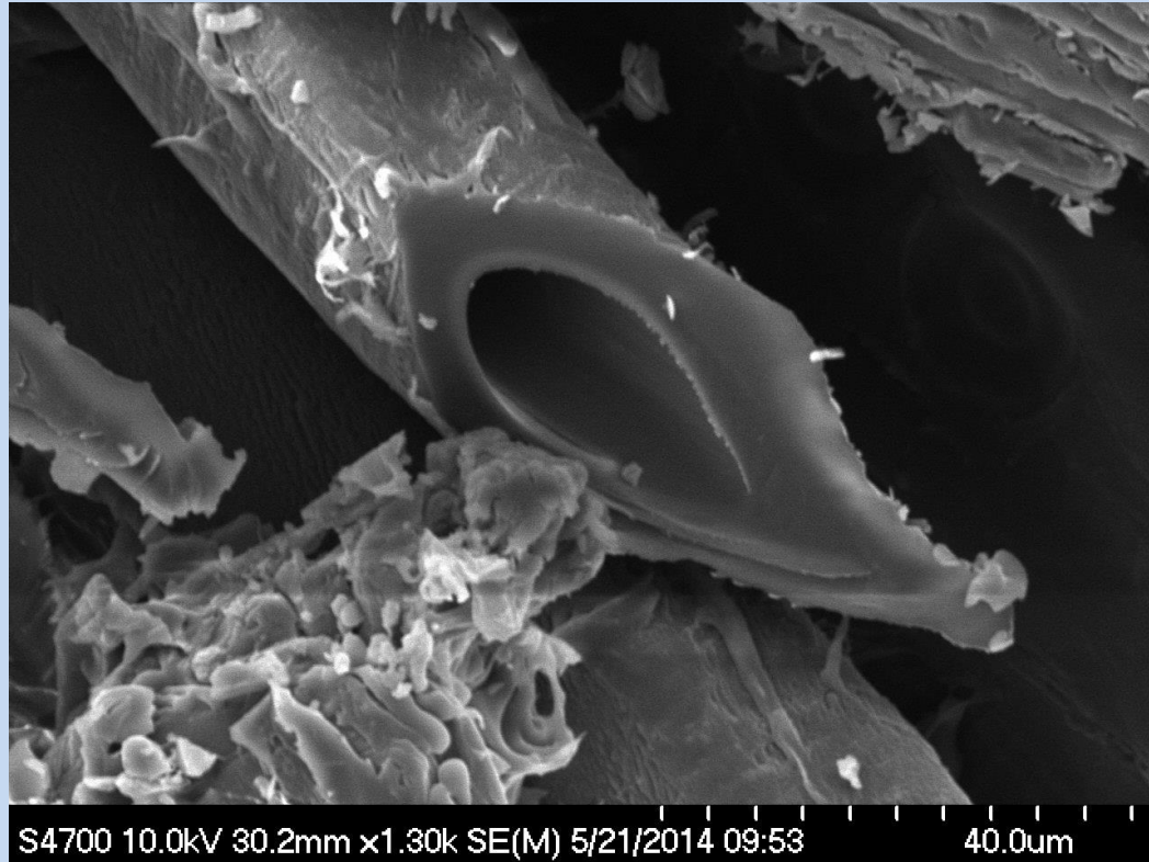
Single conduit from ruptured Douglas fir
