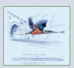
The shape of the nose of this high-speed train is mirrored by the beak of the kingfisher. The kingfisher's beak is very much streamlined. Because of this, there are no ripples on the water when the bird dives to catch a fish from the water. As the nose of the train is just as streamlined as the kingfisher's beak, the train is quieter and uses less energy.
